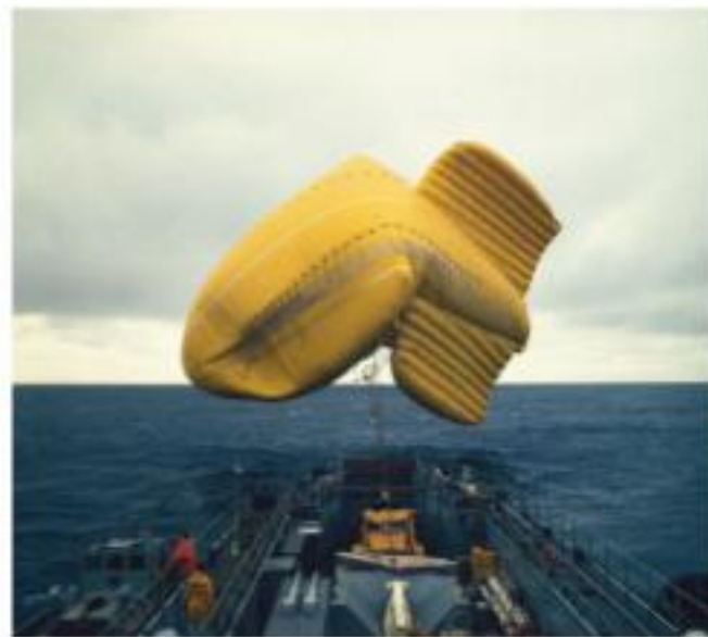
Avarie de ballon due aux conditions climatiques.
